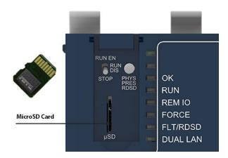
**Note:** the MicroSD Card needs to be inserted in the slot with the correct orientation. The pins of the card need to face towards the front of the equipment.
