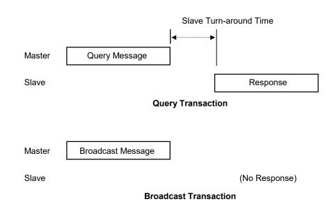
The master device begins a data transfer by sending a query or broadcast request message. A slave completes that data transfer by sending a response message if the master sent a query message addressed to it. No response message is sent when the master sends a broadcast request.
