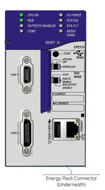
Figure 17: External Features of CPE302/CPE305-Bxxx
