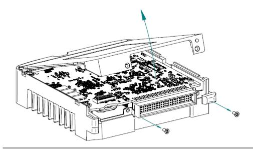
7. Open the module's cover to expose the circuit board and coin battery.
