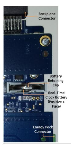
The CPE330 is shipped with a real-time clock (RTC) battery installed (see Figure 24). There is no isolation barrier between the battery and the circuit. This battery will need to be replaced periodically. Typically, no action is required during initial installation.
