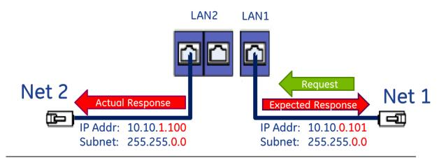
The issue demonstrated in Figure 41 is that requests entering one CPE330 interface can be routed out the other interface since both CPE330 Ethernet ports have been configured to be on the same network (255.255.0.0) but are physically connected to separate networks. Avoid this by assigning non-overlapping Subnets.
