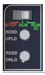
The RDSD and RUN/STOP Switches are located behind the protective door, as shown in Figure 11. Refer to
