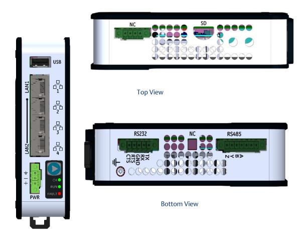
The PACSystems RSTi-EP EPSCPE100/CPE115 are enhanced performance standalone programmable controllers equipped with 1MB of user memory and four Ethernet ports to run real-time deterministic control applications. LAN1 is dedicated to high-speed Ethernet and LAN2 is comprised of three
